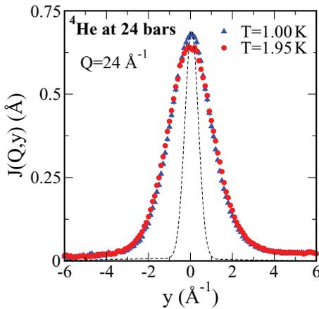
FIG. 2. (Color online) Observed  $J(Q, y)$  at  $Q = 24 \text{ \AA}^{-1}$  and at the temperatures indicated. The black dashed line is the measured ARCS resolution function at  $Q = 24 \text{ \AA}^{-1}$ , which has a full width at half maximum (FWHM) of  $0.76 \text{ \AA}^{-1}$ . The increased peak height at low temperature is attributed to the onset of BEC.
