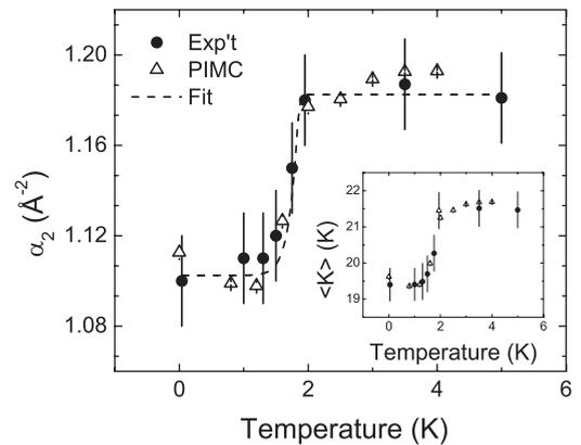
FIG. 5. Temperature dependence of the width  $\bar{\alpha}_2$  of  $n^*(\mathbf{k})$  at  $p = 24$  bars: simulation and experiment. The dashed line shows that  $\bar{\alpha}_2(T)$  has a temperature dependence that tracks  $n_0(T)$ . The inset shows the corresponding  $\langle K \rangle(T)$ .
