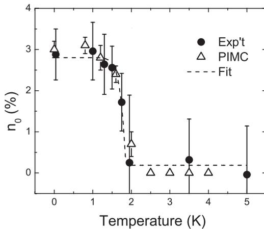
FIG. 4. Observed condensate fraction as a function of temperature. The dashed line is a line fit to the experimental data using  $n_0(T) = n_0(0)[1 - (T/T_\lambda)^\gamma]$ , where  $T_\lambda = 1.86$  K. The open triangles are the simulated PIMC results.
