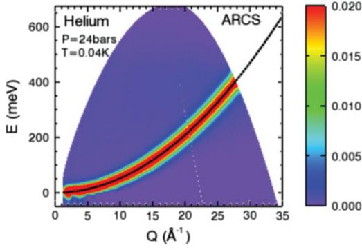
FIG. 1. (Color online) Observed scattering intensity  $S(Q, \omega)$  as a function of energy transfer  $E = \hbar\omega$  and momentum transfer  $\hbar Q$  from liquid  ${}^4\text{He}$  at  $p = 24$  bars and  $T = 40$  mK. The signal from the empty Al container has been subtracted. The black dashed line is the calculated  ${}^4\text{He}$  recoil line  $E_r = \hbar^2 Q^2/2m$ , shown as a guide to the eye.
