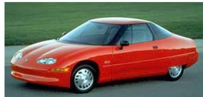
The GM Gen II EV1 is available now. It runs on 312 volts of lead acid batteries, or 343 volts of Nickel Metal Hydride batteries. With a weight around 3000 lbs, it can transport two passengers up to 130 miles. At 136 horsepower it can do 0-60 in 9 seconds, and has a top speed of 80 mph.
