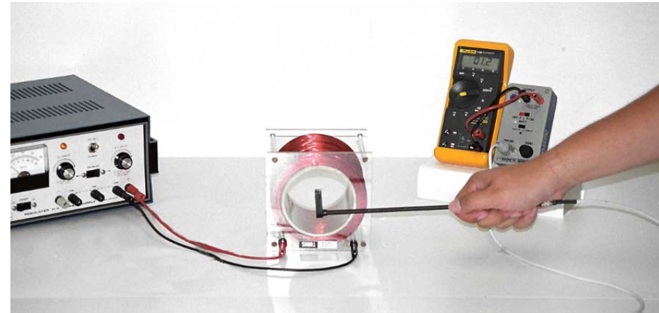
Figure: Measurement of the radial magnetic field component at the center of the coil ( s=0 ), in a plane 10cm from the center of the coil ( Z=10\text{cm} ).
